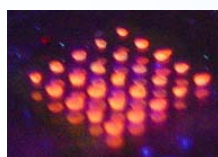
Figure 3: Photo curable polymer blends in RGB colours structured by a 5 x 5 mask with 100 micron apertures. (Under UV illumination)
