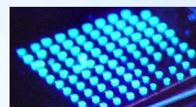
Figure 3: Photo curable polymer blends in RGB colours structured by a 5 x 5 mask with 100 micron apertures. (Under UV illumination)
